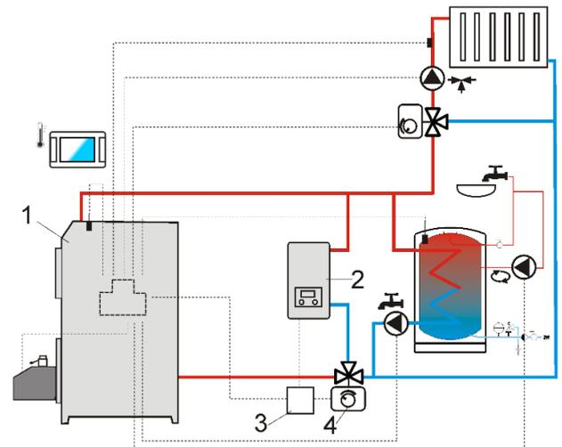
Hydraulic diagram with reserve boiler: 1 – regulator, 2 – reserve boiler, 3 – relay, 4 – switching valve (with limit switches).
