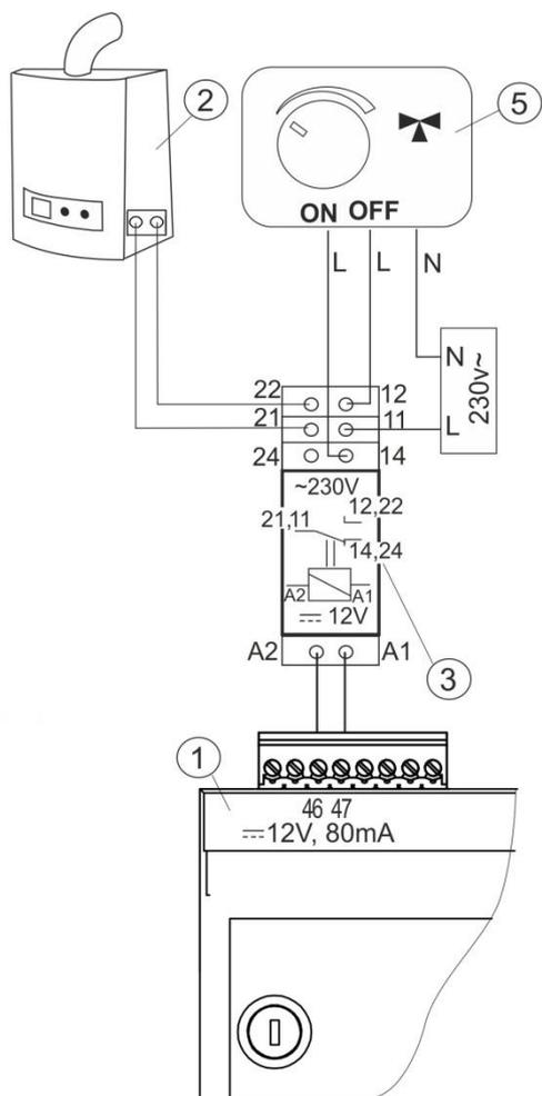
Wiring diagram of control of the switching valve in the reserve boiler: 1 – regulator, 2 – reserve boiler, 3 – relay, 5 – switching valve servo (with limit switches).
