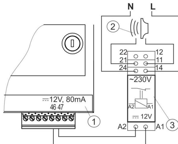
Connection of an external alarm annunciator. 1- regulator , 2 - external alarm annunciator, 3 - relay.
