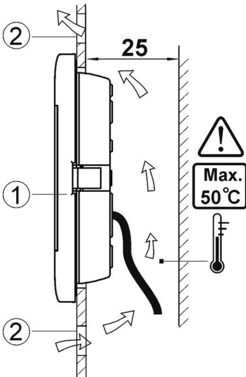
Control panel mounting requirements. 1 - control panel, 2 - vent holes to provide air circulation (note: the holes may not cause downgrading of required IP rating. They are not required if permitted ambient temperature around the control panel is not exceeded.)
