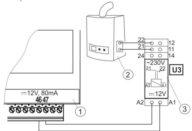
Model diagram of layout for connecting a reserve boiler to the regulator: 1- regulator, 2 – reserve boiler (gas- or oil-), 3 – relay RM 84-2012-35-1012 and base GZT80 RELPOL.
