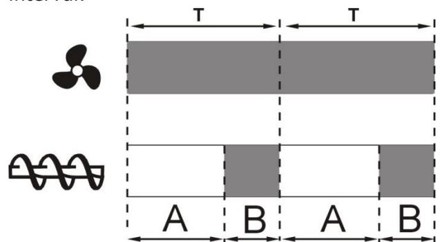
A - feeder interval, B - feeding cycle time.
