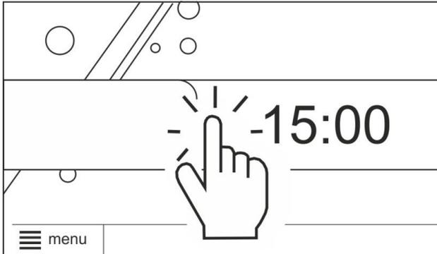
Confirm the message. Boiler enters firing-up stage.
