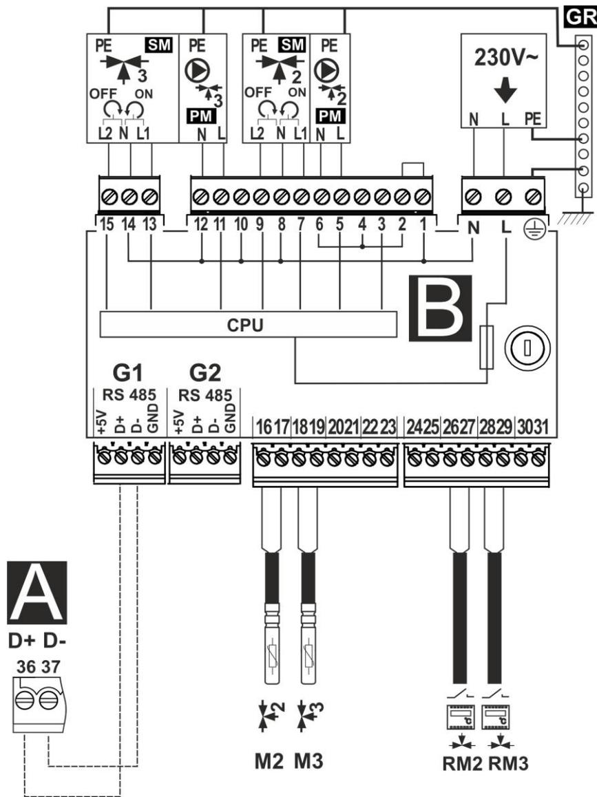
**Wiring diagram – additional B module:** **M1** – regulated circuit (mixer 2) sensor temperature type CT4, **M2** – regulated circuit (mixer 3) sensor temperature type CT4, **RM2** – mixer 2 room thermostat, **RM3** – mixer 3 room thermostat.
