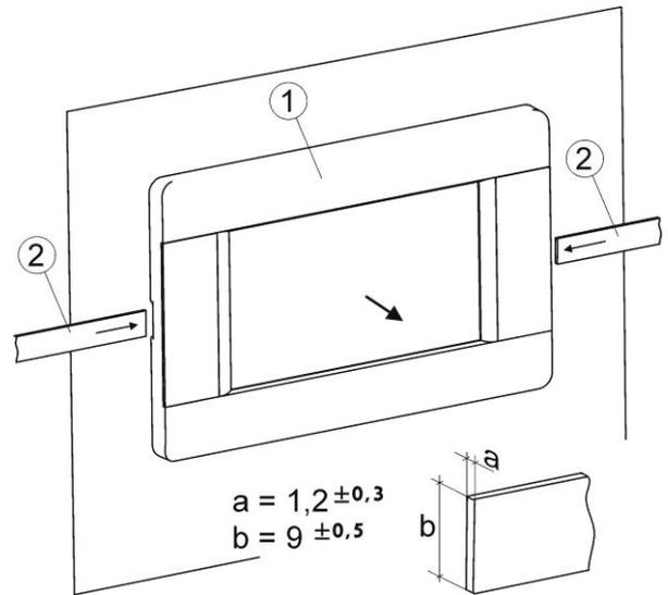
To remove the control panel (1) from the housing - insert flat elements (2) into indicated slots to release housing catches and remove the panel (1).
