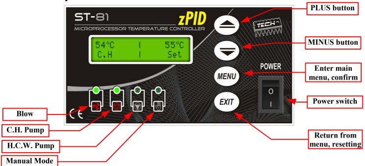
The **ST-81zPID** temperature regulator is intended for use with central heating boilers. The regulator is used for controlling the central heating water circulation pump, hot consumption water pump and blow (fan).
