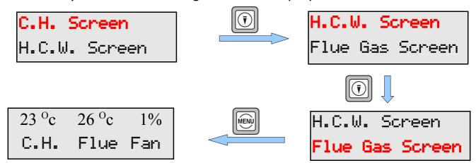
The left of the screen shows the boiler temperature; the middle of the screen shows the flue gas outlet temperature; the right of the screen shows the power of the fan. Press EXIT to return to the main menu.
