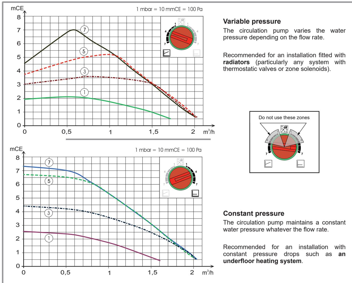
figure 30 - Available hydraulic pressures and flow rates
