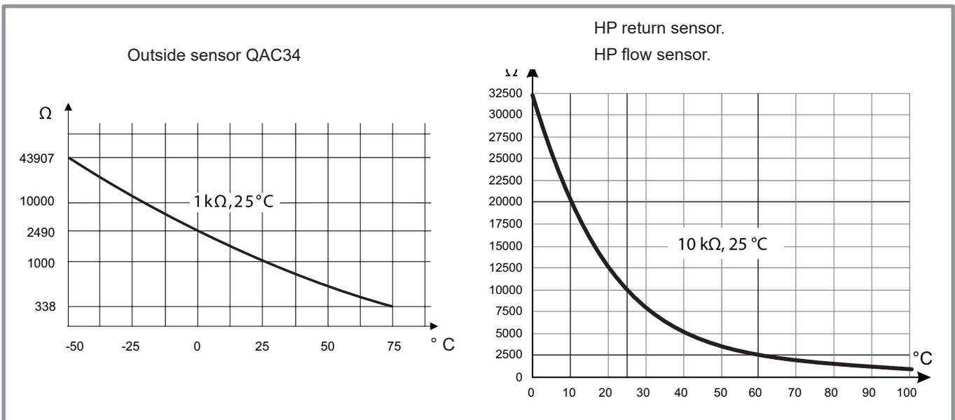
figure 6 - Ohmic sensor values (Hydraulic unit)
