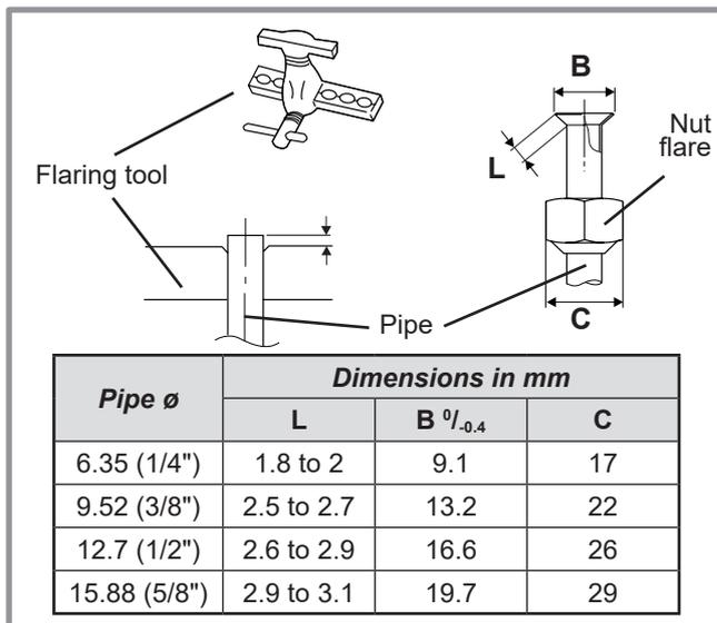
figure 18 - Flaring of the flared connections
