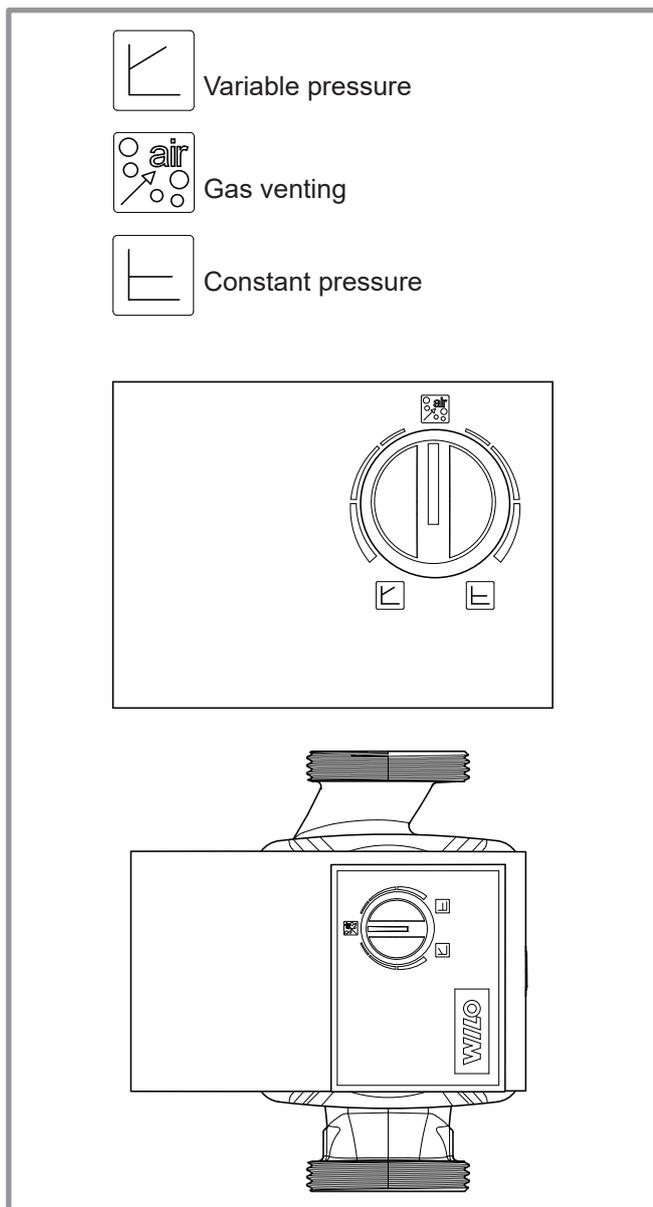
figure 32 - Circulation pump control button
