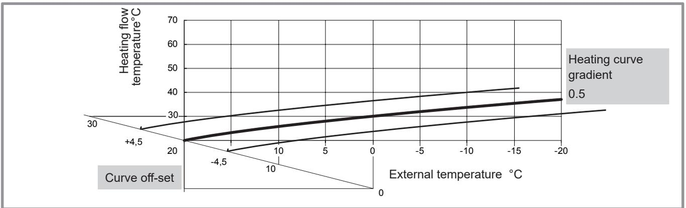
figure 43 - Transferral of the heating curve
