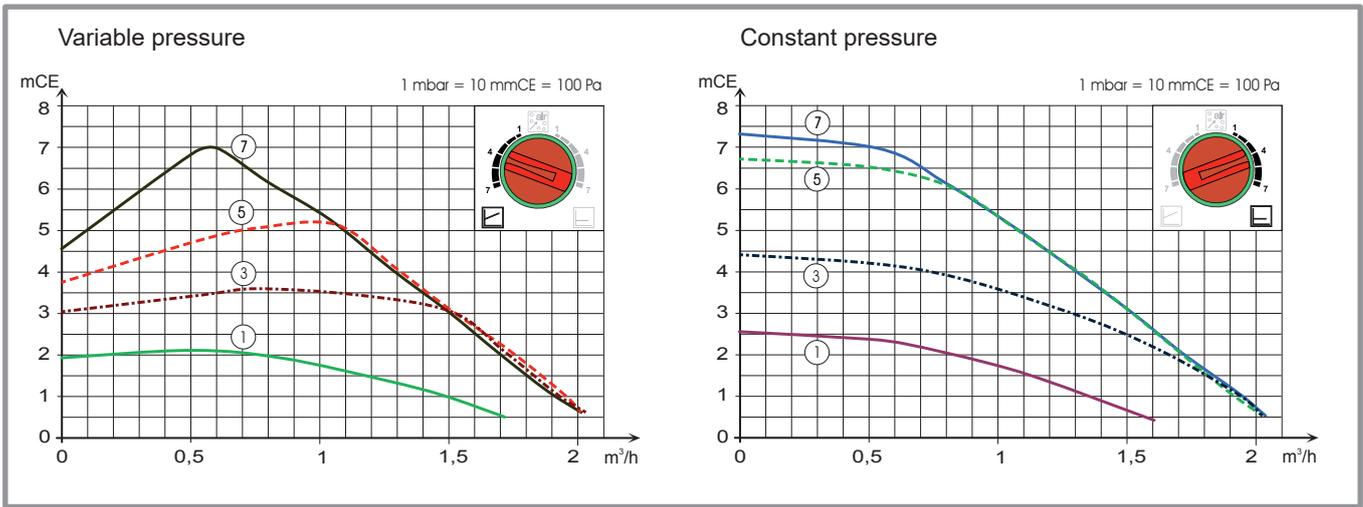
figure 5 - Available hydraulic pressures and flow rates
