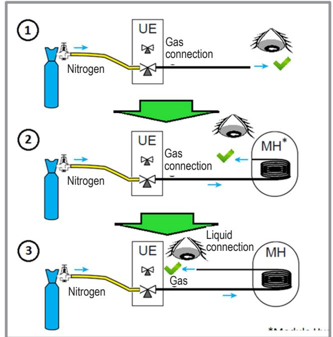
figure 21 - Checking refrigeration connections
