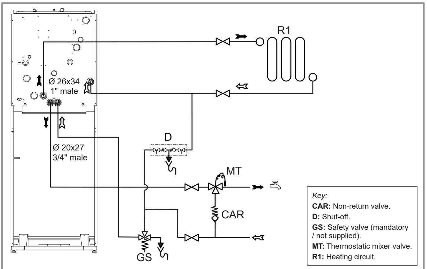
figure 25 - Basic Hydraulic Layout
