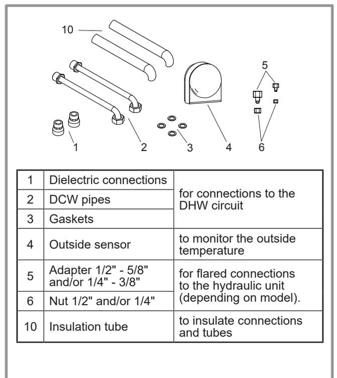
figure 4 - Accessories provided with the hydraulic unit
