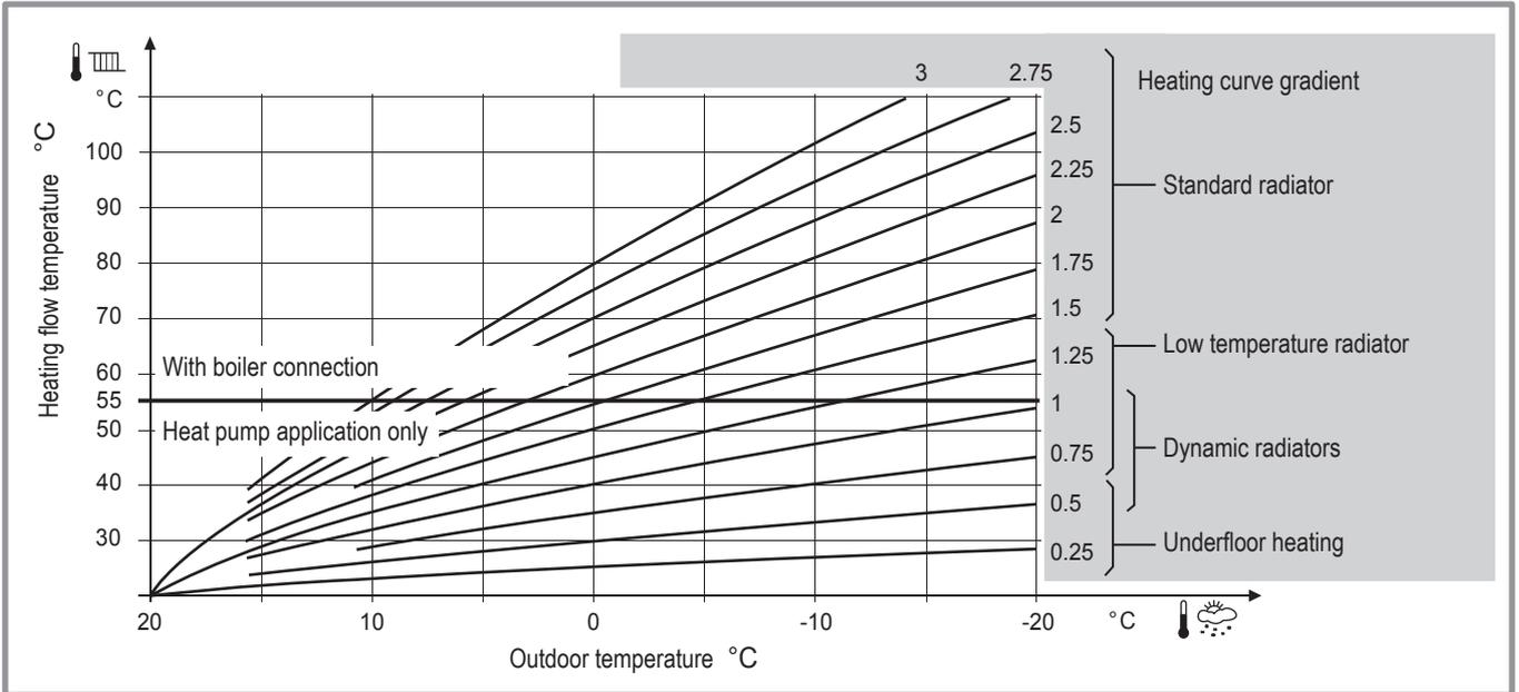
figure 42 - Heating curve gradient
