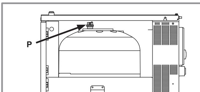
figure 29 - Hydraulic unit automatic bleeder valve
