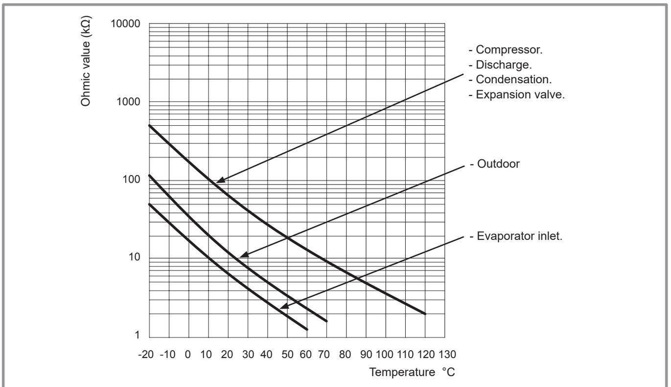
**figure 7 - Ohmic sensor values (Outdoor unit)**
