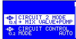
**13.1 Circulation mode 2** – This parameter allows you to attach the second circuit, and choose whether this mode is to be operated stirrer with a pump or the pump itself.
