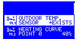
**14.1 Outside temperature sensor** – if the system is equipped with an external temperature sensor, this parameter allows you to specify whether the sensor is installed. In the absence of this parameter the sensor has to be turned off.
