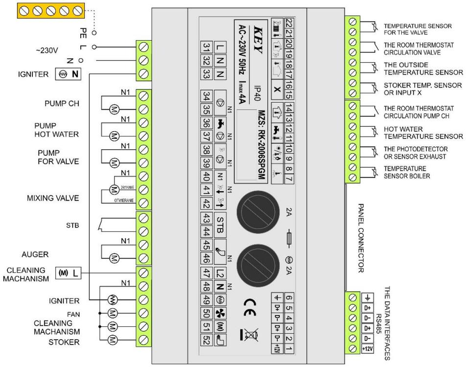
Figure 2. RK-2006SPGM+MZS Controller connection diagram.
