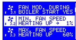
**3.1 Fan modulation during boiler start** – selection of „YES” setting means that fan speed modulation will be provided during boiler start.
