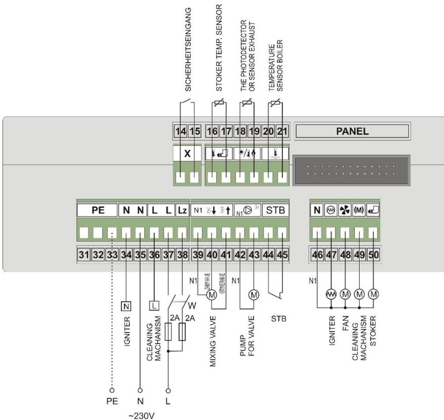
Figure 3. RK-2006SPGM+MZL Controller connection diagram.
