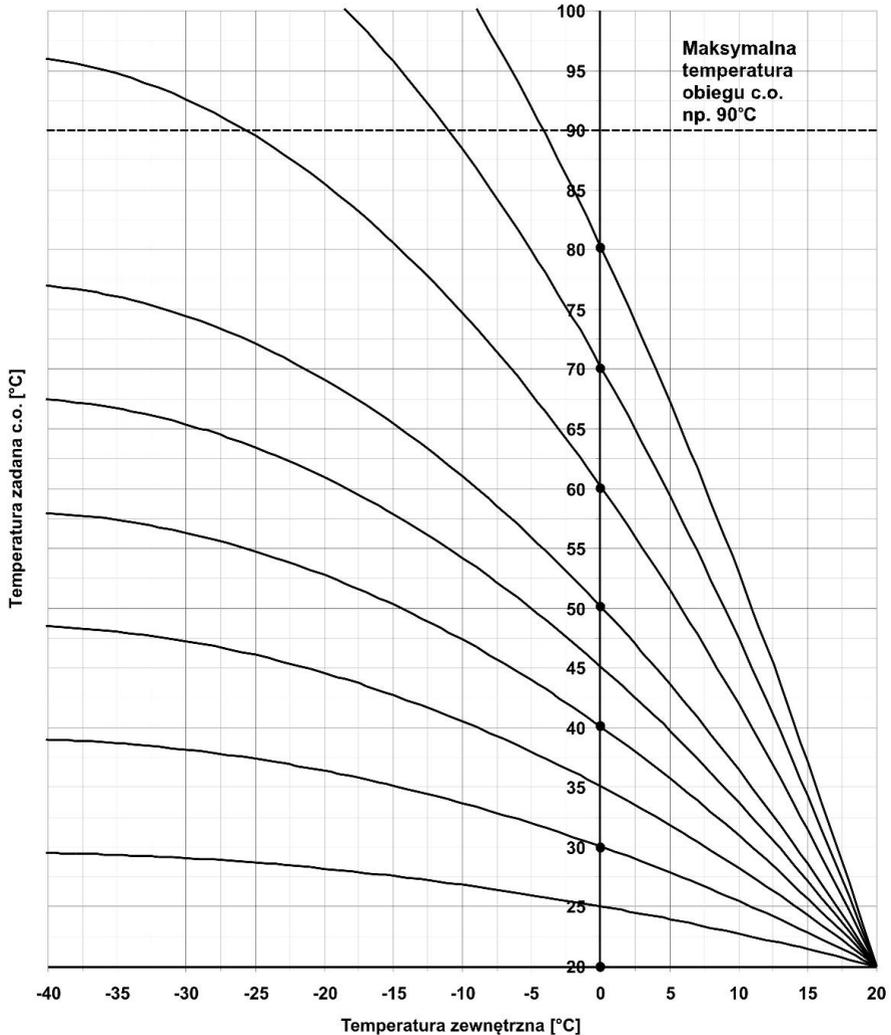
**The ratio of weather characteristics inclination** – the parameter defines the CH water temperature, when the outside temperature is 0. The relation between the outside temperature and the CH circulation water temperature for ten exemplary settings of the parameter is shown in the graph.
