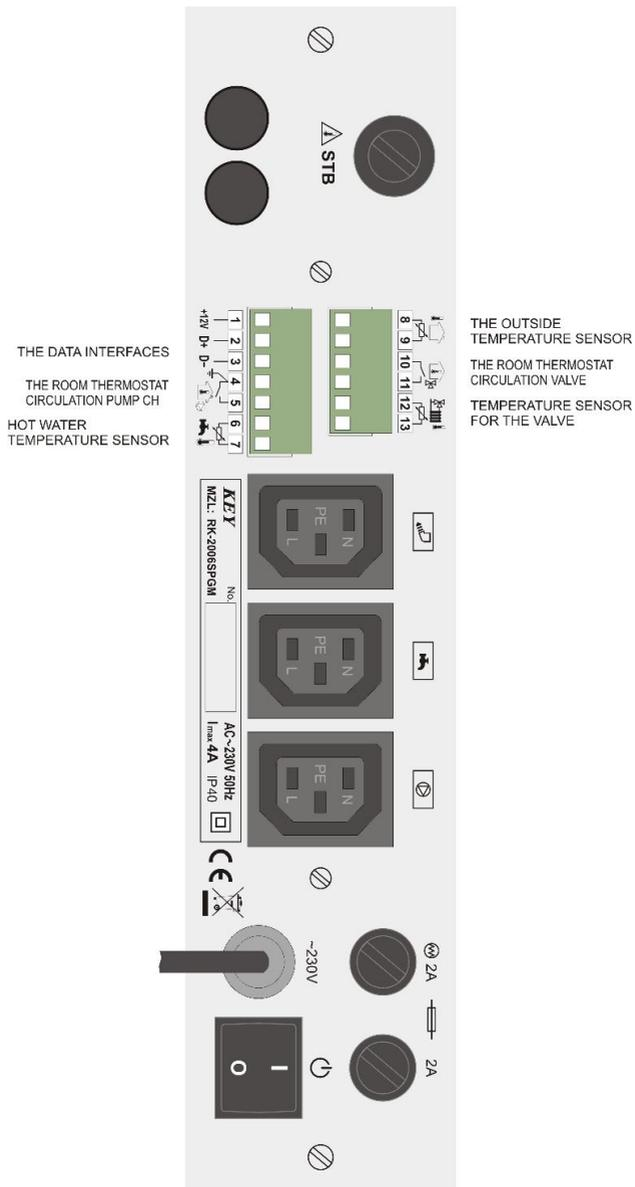
Figure 4. RK-2006SPGM+MZL Controller connection diagram.
