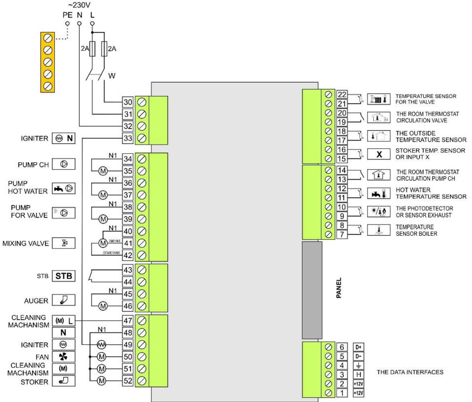
Figure 1. RK-2006SPGM + MZK, MZM2 Controller connection diagram.
