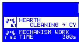
**6.1 Furnace cleaning mode** – this parameter specifies the way the cleaning mechanism works:
