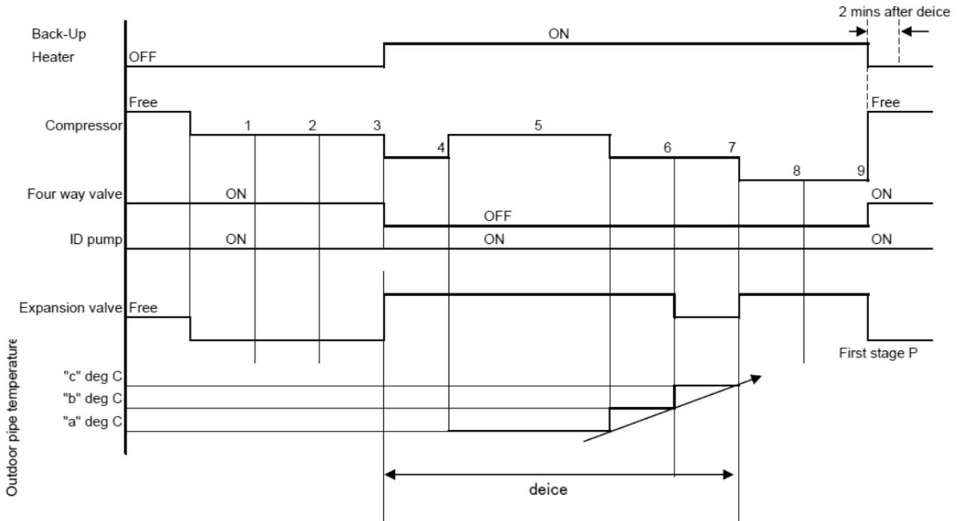
\* Backup heater must Turn OFF if the water pump turn OFF.
