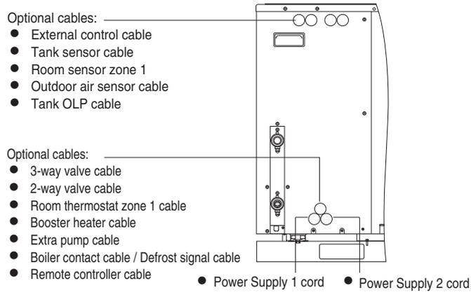
How to guide optional cables and power supply cords to Bushing ⑮
