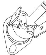
Use test pen to push this button for reset Overload Protector ⑩.
