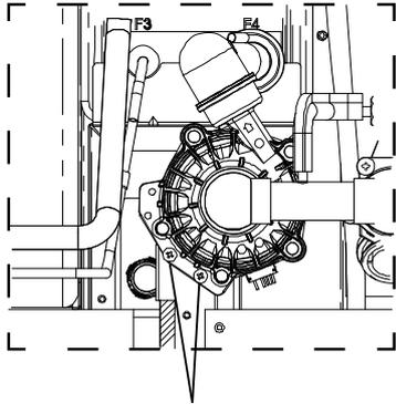
2. Remove 2 screw from Pump Bracket.
