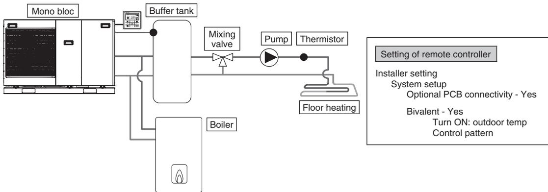
This is an application that connects the boiler to the Mono bloc, to compensate for insufficient capacity by operate boiler when outdoor temperature drops & heat pump capacity is insufficient.
