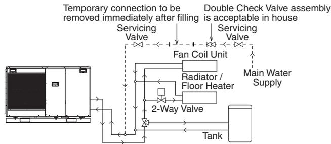
Please engage a licensed water circuit installer to install this water circuit.
