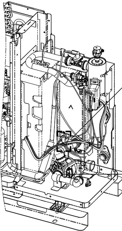
3. Remove 2 retaining ring, then slowly pull out the water pump.
