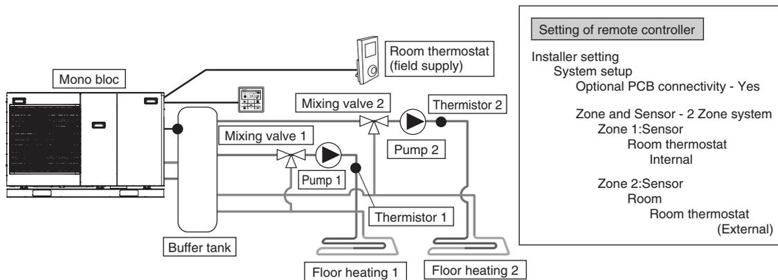
Connect floor heating to 2 circuits through buffer tank as shown in the figure.
