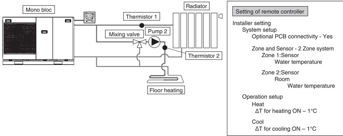
This is an example of simple 2 zone control without using buffer tank.
