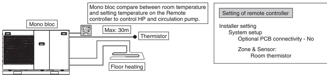
Connect floor heating or radiator directly to Mono bloc.
