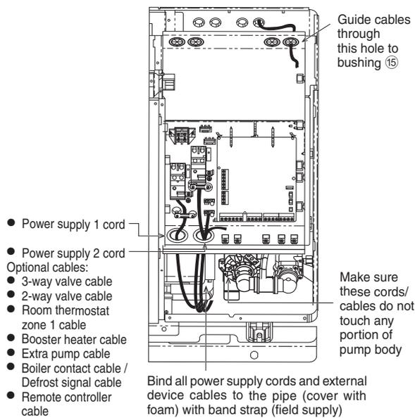
How to guide optional cables and power supply cords to control board
