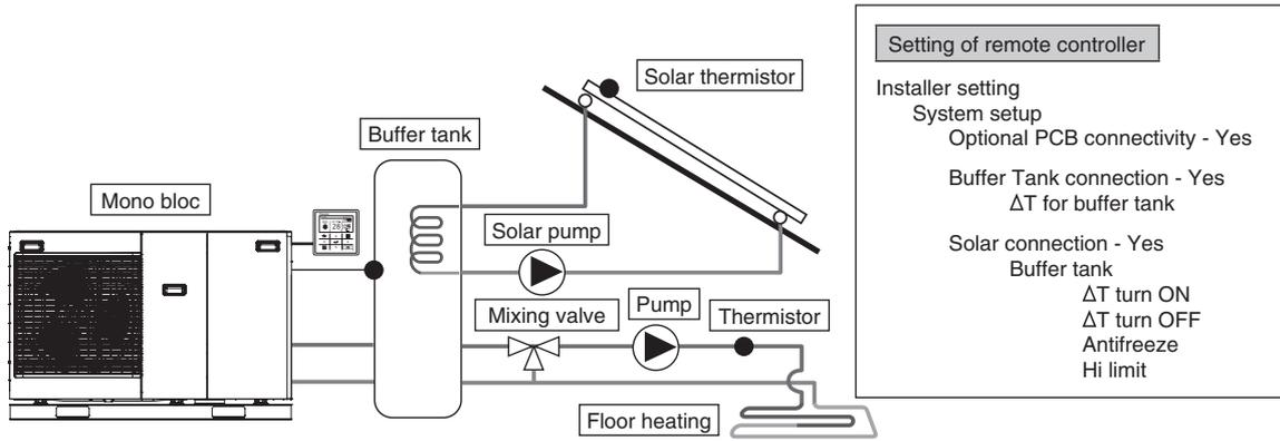
This is an application that connects the buffer tank to the Mono bloc before connecting to the solar water heater to heat up the tank.
