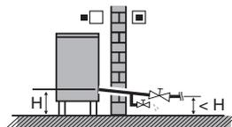
When water is idle inside the system, freezing up is very likely to happen which could damage the system.
