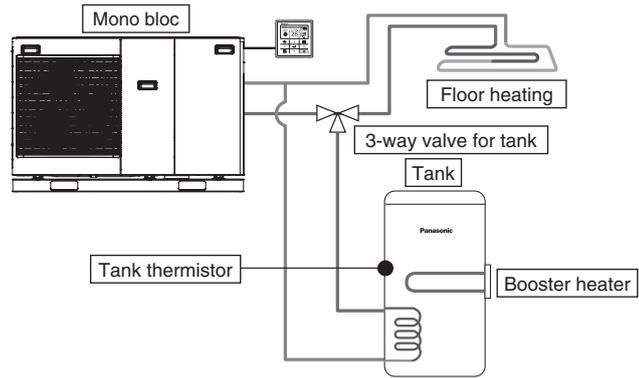
This is an application that connects the DHW tank to the Mono bloc through 3-way valve. DHW tank's temperature is detected by tank thermistor (specified by Panasonic).
