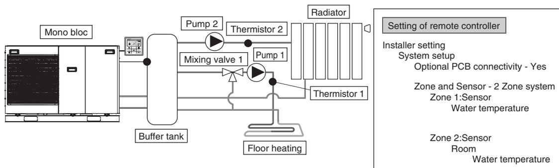
Connect floor heating or radiator to 2 circuits through buffer tank as shown in figure.
