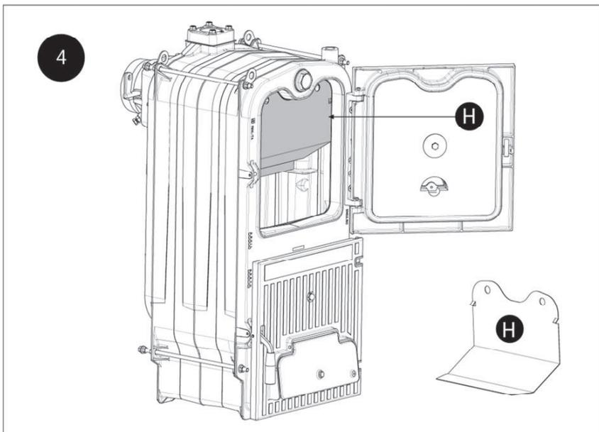
Unpack parts of convertible kit. Check if the composition agree with the size of the boiler. Check if the concrete parts are not damaged.
