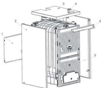
Two superior tie rods are screwed on three nuts at the front side of the boiler: the second and the third nut serve to place correctly the lateral sides of the casing. Two nuts, one for fixing the clamp holders for the lateral sides are screwed on the inferior tie rods, both from the front side and from the rear side. The assembly of the casing components has to be carried out in the following way:
